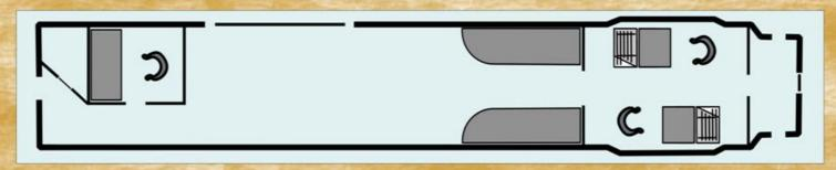
After the restoration, a special compartment was built for the train master and a luggage compartment within which there is some space for a radio cabin and an electric generator feeding the train.
