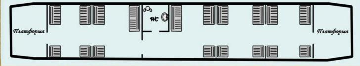
After its restoration, this railcar preserved its initial capacity of a total of 27 third-class seats. The seats are arranged according to the 2+1 scheme.
