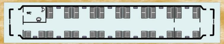
After its restoration, this railcar preserved its initial capacity: 6 second-class seats and 32 third-class seats, or a total of 38 seats. They are arranged according to the 2+1 scheme. The railcar has a toilet and a steam heating section.
